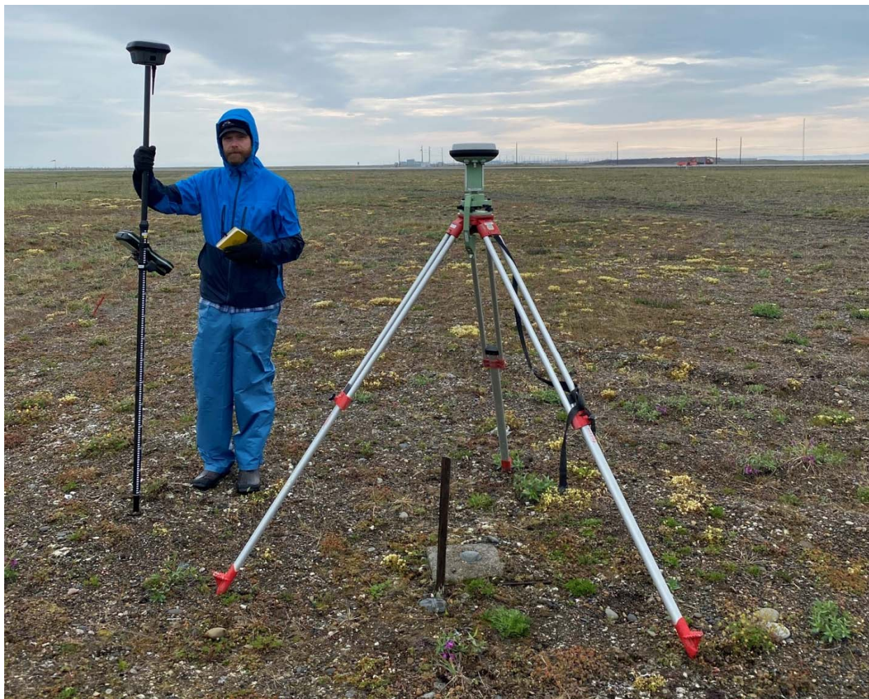
Figure 3. Survey base station and rover, held by Sean Burkholder, setup on the sole National Geodetic Survey benchmark near Point Hope. The real time kinematic (RTK) global navigation satellite system (GNSS) equipment is required to accurately survey locations and elevations of critical features and to ground truth drone and satellite imagery. Photo taken by Christopher Small on 19 July 2021. IMG_3543.jpg.
